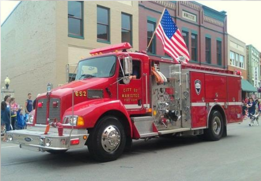
Engine 652 – 2004 Pierce Pumper 1250 GPM pump
